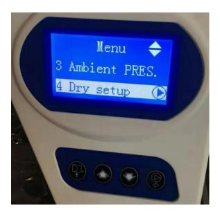
The initial data is 30, then you can change it to 35, press up key adjust, then confirm, if still wet, change to 38...
