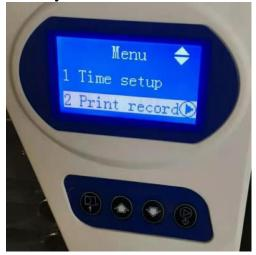
Up —down to choose, 1 means the last one record, 2 means the last 2 records, it can make a record with many times.....
